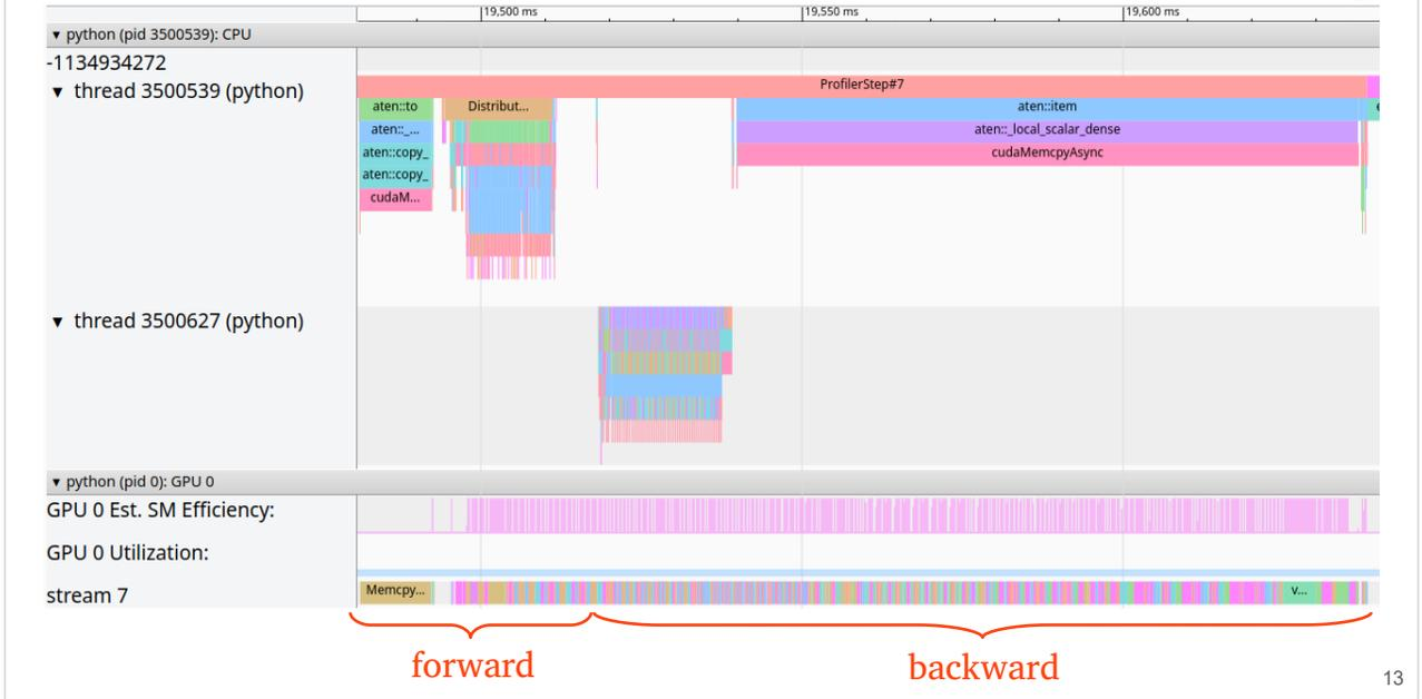
By zooming in on the part of the iteration during which the GPU is active, we differentiate the forward and backward steps.
